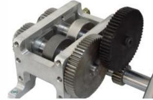
**PennyRoller's** dies are easily removable and can be swapped to respond to a particular event. Therefore, this operation requires unmounting the elements that are preventing access to dies. The dies have been heat treated to increase steel hardness, in order to resist the very high operating pressures. Each die can receive up to 4 imprints, increasing the machine's return.
